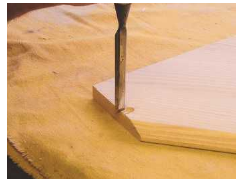
▲ Pic.20 Remove most of the waste with a brad-point drill, then trim out the rest with a sharp chisel
